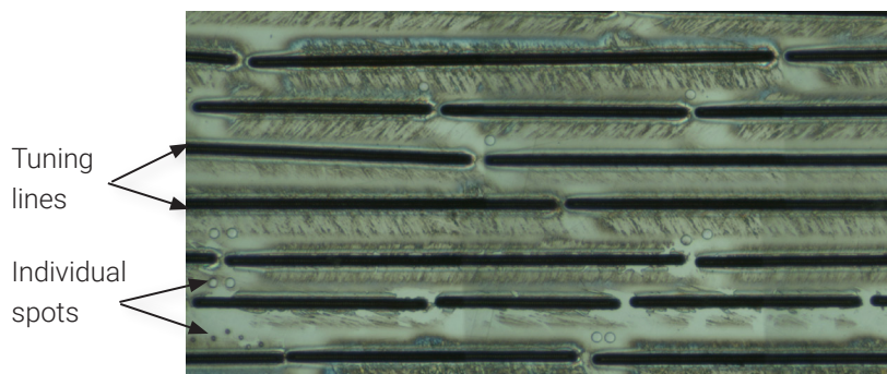
Figure 1. Ablation lines and spots in NIST 612 Glass, used for LA-ICP-MS tuning. Image courtesy of Maxwell Morrisette, CODES Analytical Laboratories, University of Tasmania, Australia.
