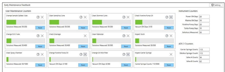
Color-coded alerts address common reasons for service calls, such as poor precision due to worn pump tubes, or poor sensitivity due to a dirty ion optics or cone interface. By alerting the analyst of a problem and then guiding them through the process of fixing it, the expense and downtime of a service call can be avoided. MassHunter versions 5.3 and higher also monitor the statistics and use of all parameters associated with the Advanced Dilution System (ADS 2)
