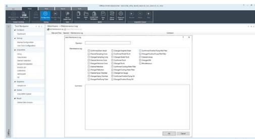
A log of maintenance activities can be generated within the ICP-MS MassHunter software.
