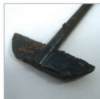
Badly damaged PTFE-coated paddle
