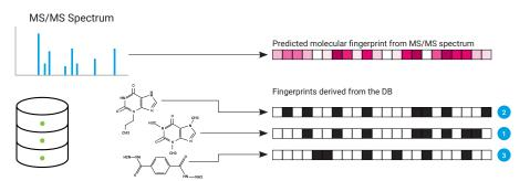
The predicted molecular fingerprint of the unknown is compared to the molecular fingerprints of structures derived from the structural DB, ranking candidates to identify the unknown.
