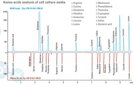
Amino acid analysis of MEM media (blue trace) overlayed with AA standard (red trace). The amino acid content of cell culture media is matching accurately with its theoretical composition.
