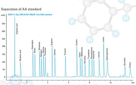
The amino acid method is used on an Agilent AdvanceBio AAA 4.6 x 100 mm, 2.7 µm column.
