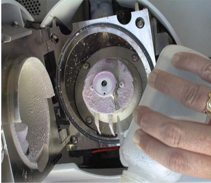
APCI-SprayChamber after 6hrs with 25mmol phosphate buffer (0.7mL/min)
