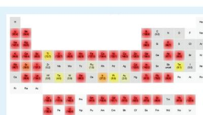
The IntelliQuant function generates a heatmap to visually represent the relative concentrations of elements present in a sample.
