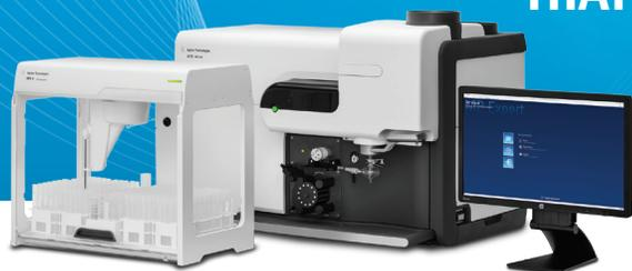
*"Agilent's MP-AES is well suited for the rapid elemental analysis of liquid samples such as wine and spirits. Because it is automated, it is easy to load and use, and frees-up valuable staff time with its walk-away platform.*
