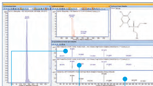
Top: Auto MS/MS spectrum Middle: Mirror spectrum Bottom: Library spectrum
