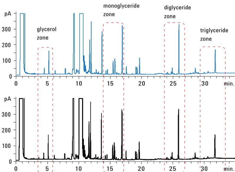
The **top** chromatogram depicts a single run of a B100 sample prepared using Agilent’s 7696A Sample Prep WorkBench. Each zone for glycerol and glycerides quantification is outlined in red. The **bottom** chromatogram overlays 10 separate samples prepared using the 7696A Sample Prep WorkBench.
