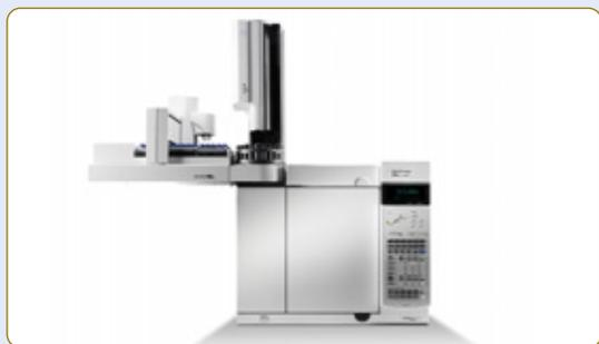
Agilent's 7890A GC gives you advanced separation capabilities, powerful new productivity enhancements, and real-time self-monitoring instrument intelligence. 5th-generation Electronic Pneumatics Control (EPC) and digital electronics set a new benchmark for pressure set-point and retention time locking precision (0.001 psi).
