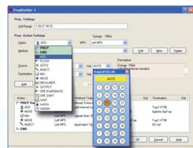
The SPE system is controlled by the GERSTEL MAESTRO software. All parameters for the various SPE steps are entered by mouse-click in the GERSTEL PrepBuilder. A link to the Agilent MassHunter Software, which controls the LC/QQQ system and the Data Acquisition, is implemented in MAESTRO Configuration Editor. The Injection volume of the SPE eluate, the MassHunter LC/QQQ method and the MassHunter Data Folder can be specified in MAESTRO without additional entries in the MassHunter software.
