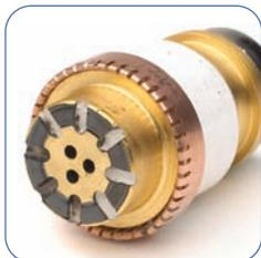
**A high performance triple-axis detector** that uses an ion guide and shield to position a triple-channel electron multiplier doubly off-axis from the analyzer exit. This optimized path increases the signal and eliminates noise from energetic neutrals.
