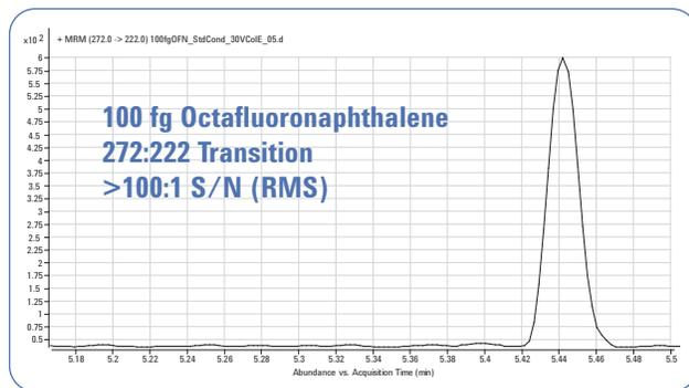
**Shattering the barriers of sensitivity:** In this example, the Agilent 7000A Triple Quadrupole GC/MS detected 100 fg of Octafluoronaphthalene at greater than 100:1 signal-to-noise ratio.
