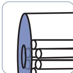
**Patent-pending collision cell design:** The linear acceleration design of Agilent's 7000A Triple Quadrupole GC/MS is optimized for high-speed performance without ion ghosting or cross-talk. In addition, speeds of up to 500 MRM per second allow you to determine more compounds per ion group, while a wide mass bandwidth optimizes sensitivity by eliminating the need to tune on your compound.
