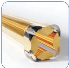
**A gold-standard quadrupole design with exceptional dimensional stability:** Temperature changes up to 200° C will not alter the quartz dimensions of Agilent's single-piece, gold-plated analyzer. This high-temperature stability ensures superior mass analyzer performance and also allows maintenance-free operation – even with complex, high boiling samples.
