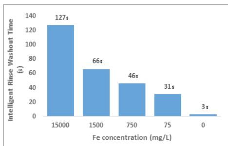
The Agilent Intelligent Rinse function adjusts rinse time, based on the time taken to wash out each element in your sample. In this example, Intelligent Rinse saved over two minutes of unnecessary rinse time when measuring samples at the low end of the calibration compared with those at higher concentrations.
