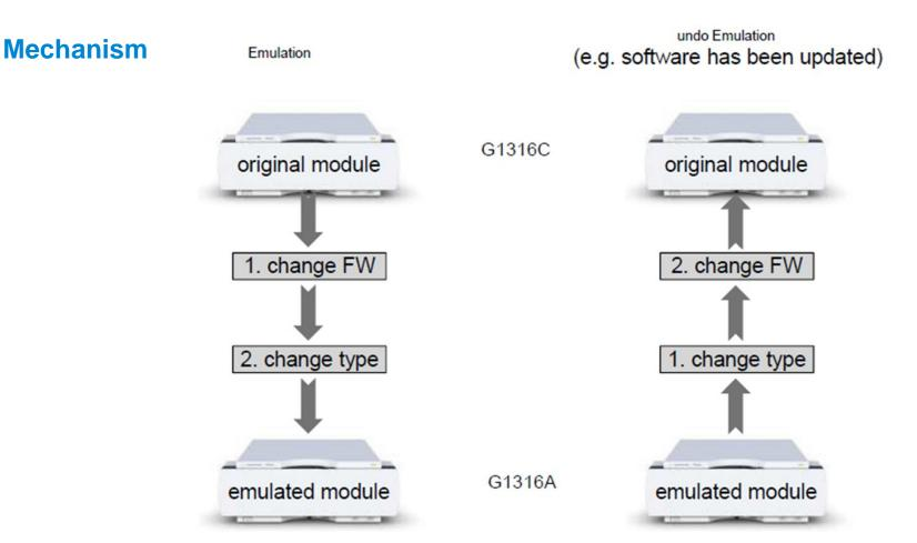
Note: if you need to update the firmware on an emulated module, e.g. G1316C emulated to G1316A or G1316B – you need to bring the module back to the original type to update the firmware.
