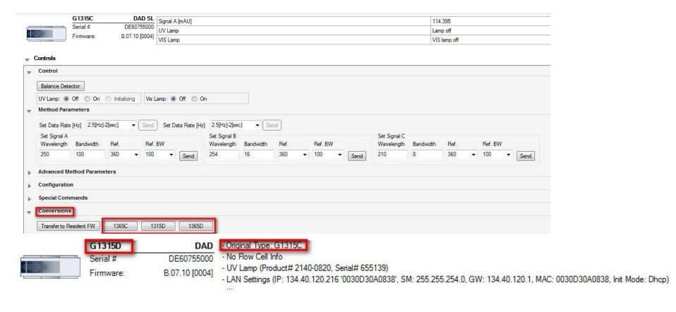
LabAdvisor will only display valid emulations. The emulated module only simulates a different model number. Internally the so called "original type" (= otype) always remains, so a quaternary G1311B pump, which is emulated to G1311A, will always use G1311B firmware.
