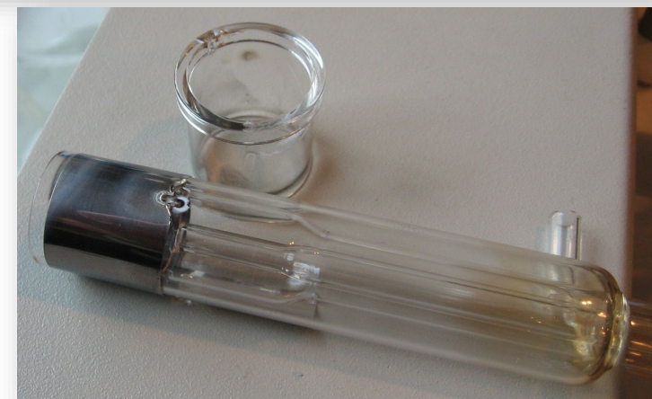
Torch damage due to incomplete drying
