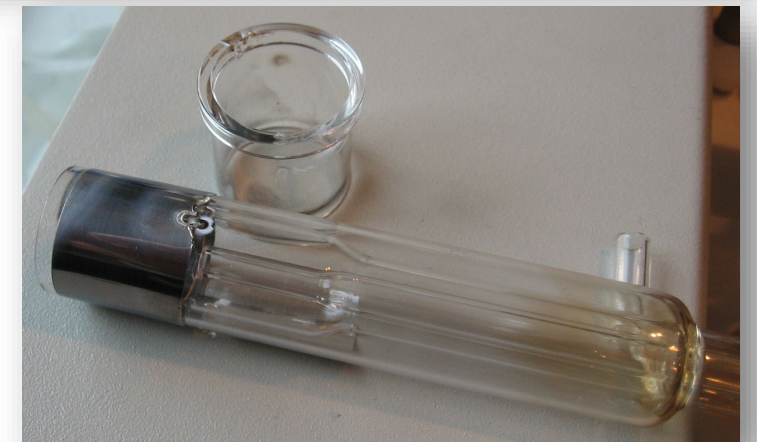
Torch damage due to incomplete drying
