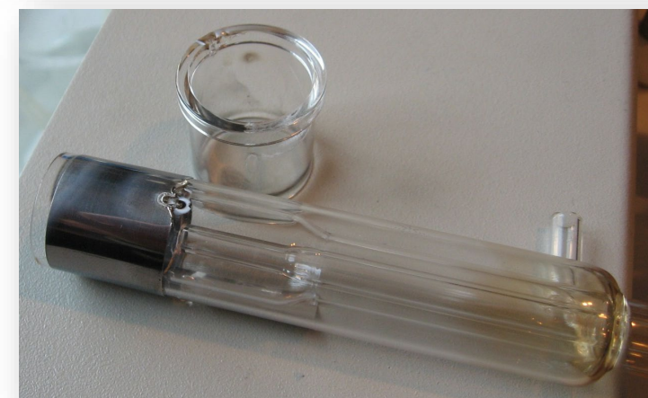
Torch damage due to incomplete drying
