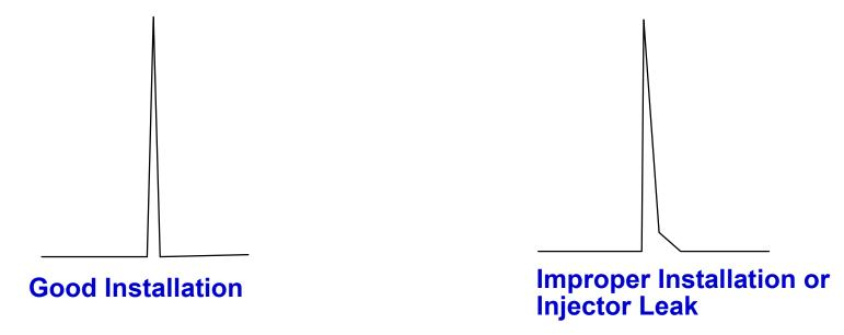
Check for: Injector or septum leak
