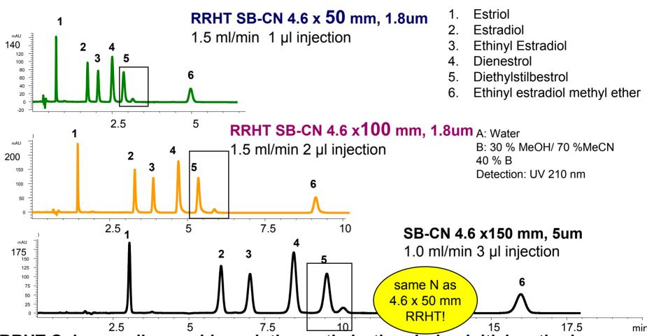
RRHT Columns allow rapid resolution optimization during initial method development. Column lengths compared quickly.
