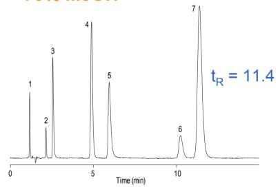
> The retention of the basic compounds in this sample increases at high pH.
