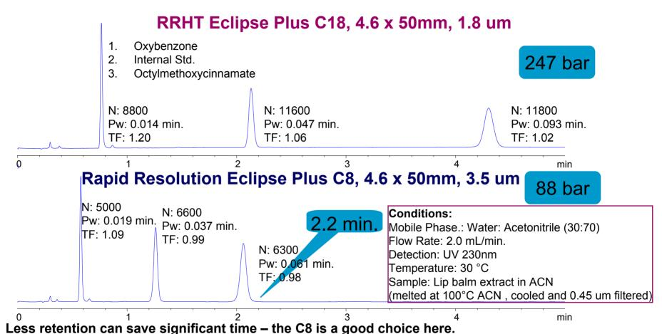
The RRHT column is delivering the efficiency and resolution expected, but the C8 bonded phase may be the better choice.
