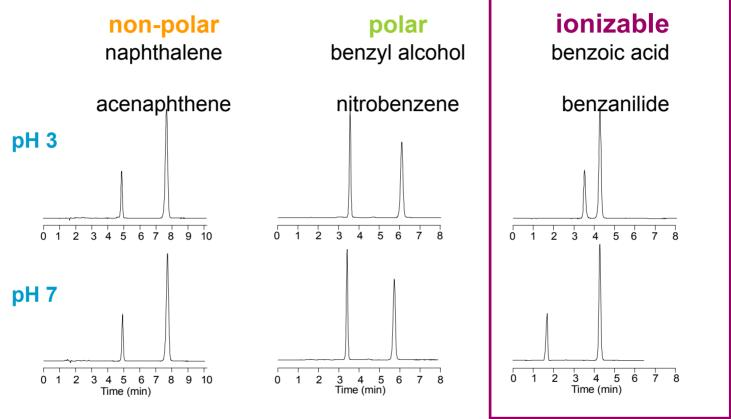
Ionizable compounds – acids and bases can change retention and selectivity the most with changes in pH
