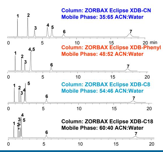
Column Dimensions: 4.6 x 150 mm, 5 μm
