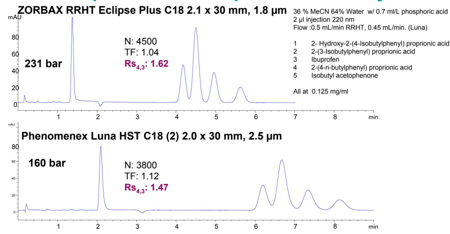
ZORBAX RRHT has at least 18% more efficiency than Luna HST C18(2) That means greater than baseline resolution when needed.
