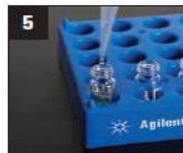
Place in autosampler vials for GC or LC analysis
