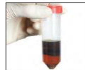
Phase separation of acetonitrile and aqueous layer
