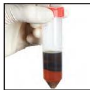
Phase separation of acetonitrile and aqueous layer
