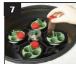
Centrifuge at 4000 rpm for 5 minutes
