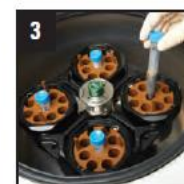
3 Centrifuge at 4000 rpm for 5 minutes
