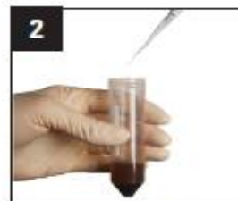
Add water and QC spikes if needed and spike with internal standard
