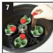
7 Centrifuge at 4000 rpm for 5 minutes
