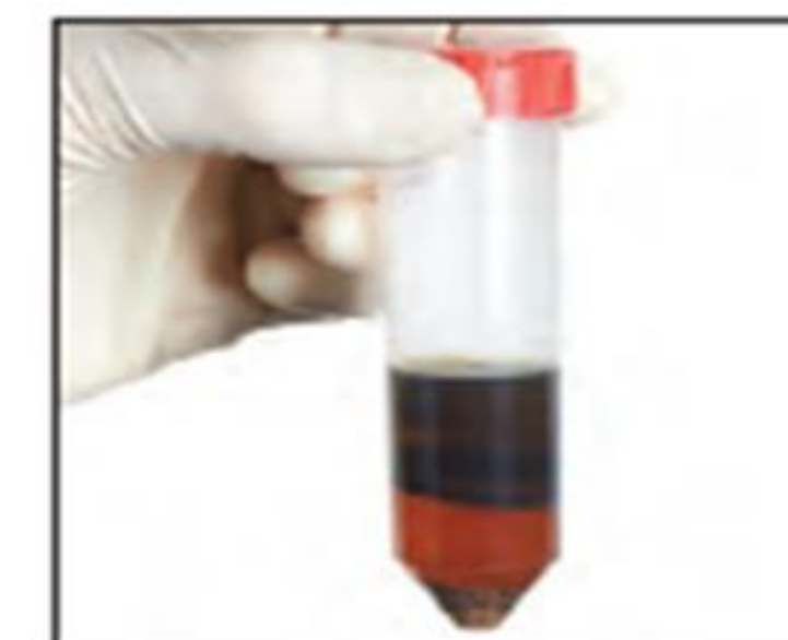
Phase separation of acetonitrile and aqueous layer
