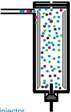
Sample expands to overfill injector
