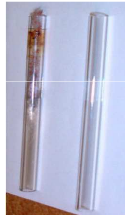
Dirty liner on left versus clean liner on right
