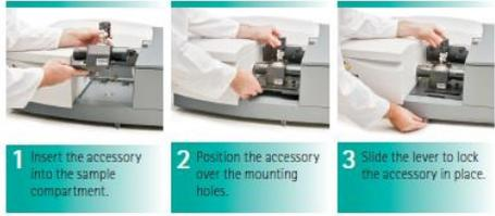
Automatic accessory recognition - identifies the accessory being used and displays relevant methods in the Method List, enabling you to run samples in seconds.
