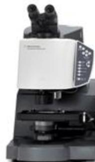
Extend the capabilities of your FTIR spectrometer with an Agilent Cary 610/620 FTIR microscope and gain new insight into areas as diverse as polymer chemistry, drug discovery, biomedical research and much more.
