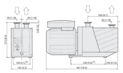
Alternative mounting holes are also available, with (1) = 226 (8.9) and (2) = 98 (3.8), with hole  $\emptyset$  = 7 (0.3)
