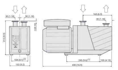
Alternative mounting holes are also available, with (1) = 226 (8.9) and (2) = 98 (3.8), with hole  $\emptyset$  = 7 (0.3)
