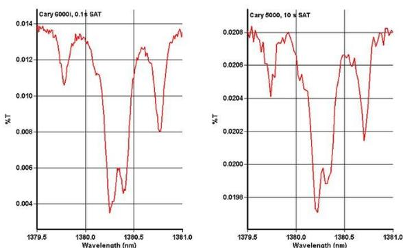
**Figure 1.** Water vapor spectrum collected on the Cary 6000i InGaAs and the Cary 5000 PbS spectrophotometers
