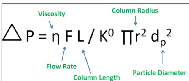
The diagram shows the pressure equation  $\Delta P = \eta F L / K^0 \pi r^2 d_p^2$  with five variables labeled in green text and blue arrows pointing to them: Viscosity ( $\eta$ ), Column Radius ( $r$ ), Flow Rate ( $F$ ), Column Length ( $L$ ), and Particle Diameter ( $d_p$ ).
