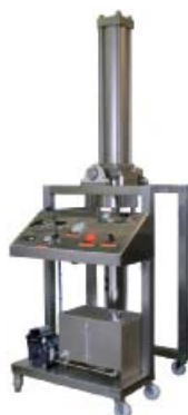
Pilot scale L&L columns - 6 in. ID
