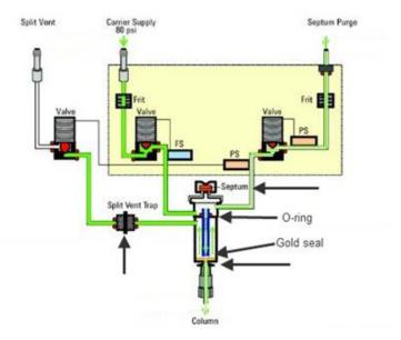
The leak check process checks for leaks in the column fitting, septum nut, weldment nut, split vent trap housing and gold seal fitting.
