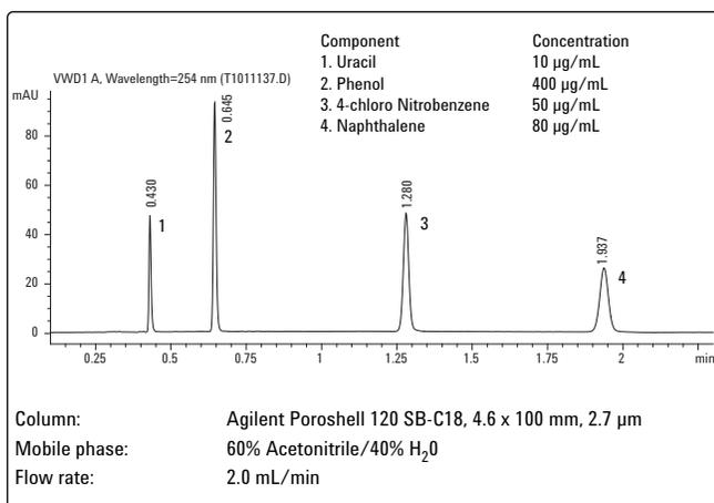
Figure 1. Agilent Poroshell 120 SB-C18 chromatogram.
