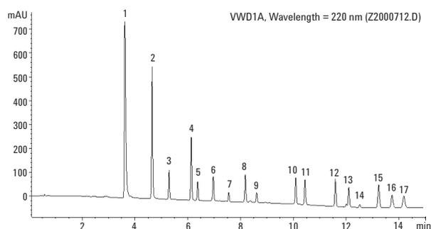
Figure 1. Agilent ZORBAX RRHD Eclipse PAH QA chromatogram.
