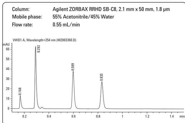
Figure 1. Agilent ZORBAX RRHD SB-C8 QC chromatogram.
