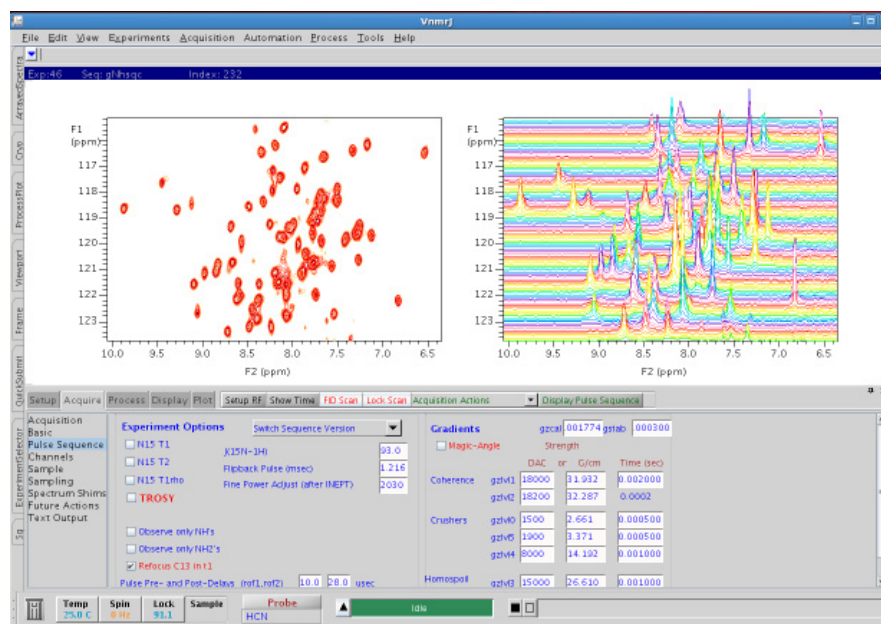
Figure 1. BioPack display of 2\text{D-}^{15}\text{N} HSQC data comparing a contour and stacked display, along with the Pulse Sequence panel showing experimental options available within the pulse sequence.
