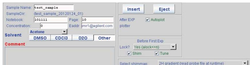
Figure 2. Automatic tuning and matching can be selected or unselected with a single click next to the **Tune** check box.
