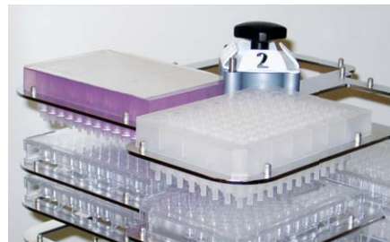
Figure 3: Cutouts in the shelves are suitable for holding filter plates.
