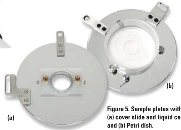
**Figure 5. Sample plates with (a) cover slide and liquid cell, and (b) Petri dish.**
