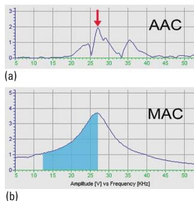
Figure 1. Typical plot of amplitude vs. frequency with AAC (top) and MAC Mode (bottom). MAC Mode operates in the highlighted frequency range and AAC operates only at the frequency indicated by the arrow.
