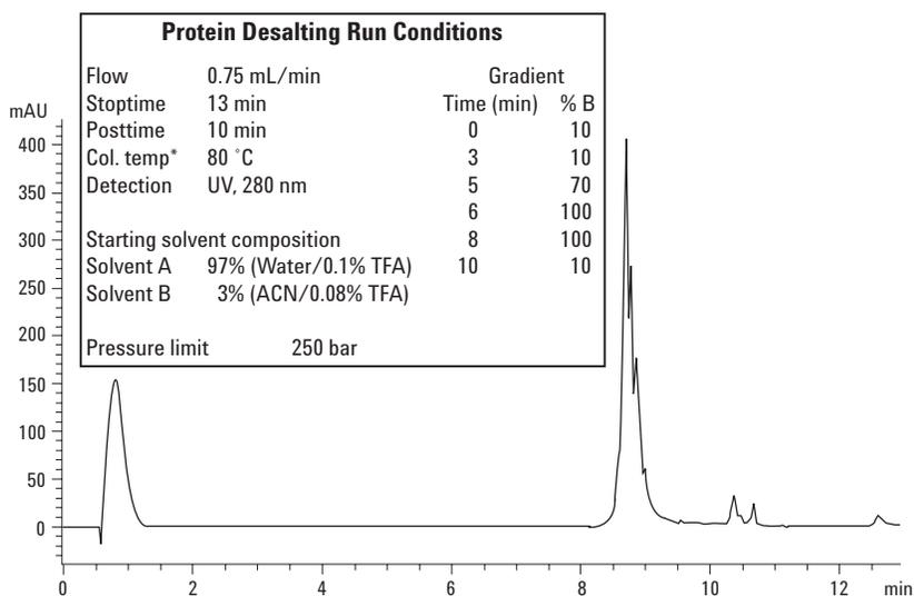
**Figure 2.** Immunodepleted serum proteins (57 µg), desalted/concentrated with optimized gradient and temperature conditions as listed with the mRP-C18 column. \*The column can be used between 70–80 °C.
