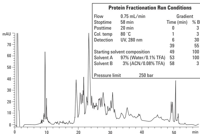
**Figure 1.** Immunodepleted human serum proteins (300  $\mu\text{g}$ ) separated on a 4.6-mm id  $\times$  50 mm mRP-C18 column at 80 °C under optimized conditions. Note that the recommended maximum amount of immunodepleted serum protein that can be loaded on this column in gradient separations is 380  $\mu\text{g}$ .
