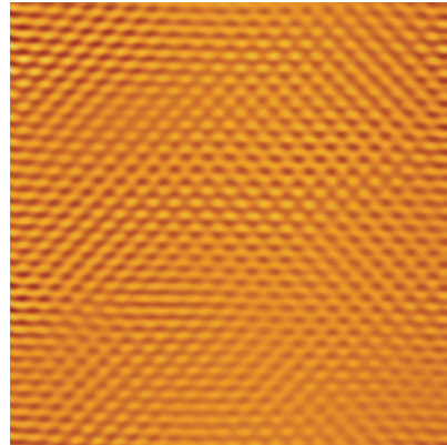
Figure 6. AFM image of mica atoms at 200°C (FFT filtered). 16nm x 16nm.
