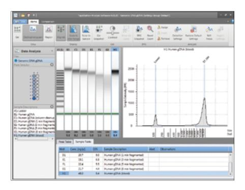
The intuitive 2200 TapeStation software represents the automatically analyzed data as a familiar gel image and electropherogram for each sample. The results are also presented in a tabular format. Additional tools are also provided for easy sample comparison and reporting.
