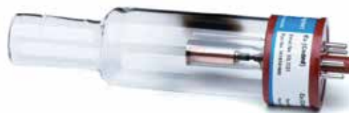
Figure 3. The black spot visible in the Agilent lamp is the active "getter" spot created deliberately to prolong lamp life and ensure continued spectral purity.
