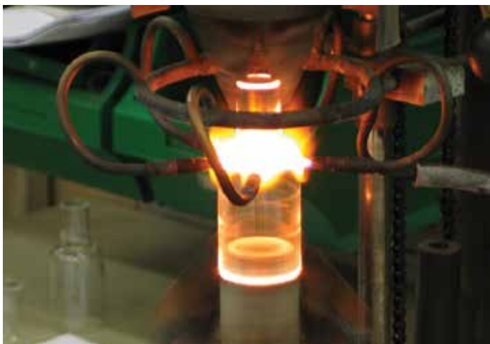
Figure 2. Agilent lamps are hand made in an ISO 9001 facility to guarantee performance and reliability. Here the graded seal is welded to the lamp base.
