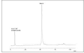
Figure 1 - HPLC of 2-AB labeled Man-8
