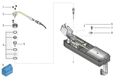
Nitrogen Phosphorus Detector (NPD) assembly (top)
