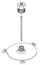
How to install glass liner on Purged Packed Inlet
