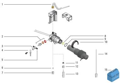
FPD ignitor and heat shield assembly
