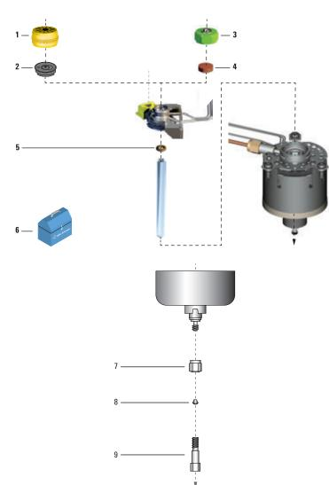
Exploded parts view of the Multimode Inlet
