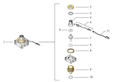
Flame Ionization Detector (FID) assembly
