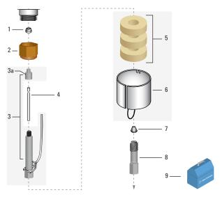
Electron Capture Detector (ECD) assembly
