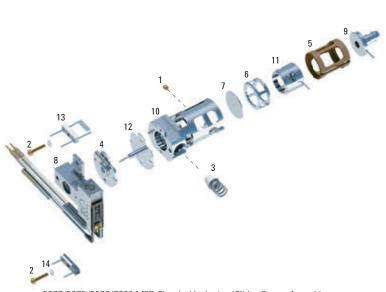
5977/5975/5973/7000 MSD Chemical Ionization (CI) Ion Source Assembly
