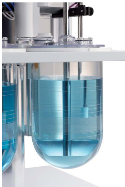
709-DS DVH 溶出杯内的非驻留取样
