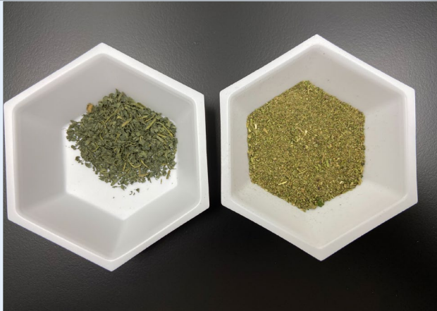
Figure 4: Comparison of manual (left) versus mechanical (right) grinding techniques.
