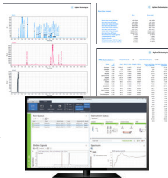
Example of OpenLab CDS reporting of light gases and hydrocarbons from an Agilent 8890 GC with FID and TCD.
