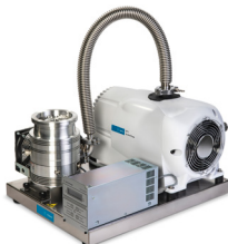
TPS-mobile turbo pumping system, TwisTorr 305 FS turbo pump, DN 100 CF-F (6 in CFF), IDP-7 scroll primary pump, no pressure gauge, US power cord
