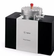
Vaclon Plus 300 L/s pump, Diode, Fischer feedthrough, DN 160 CF-F (8 in CFF), double-ended, with heaters 120 V
