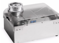
TPS-flexy turbo pumping system, TwisTorr 74 FS turbo pump, DN 63 CF-F (4.5 in CFF), IDP-3 scroll primary pump, 120 V, remote controller
