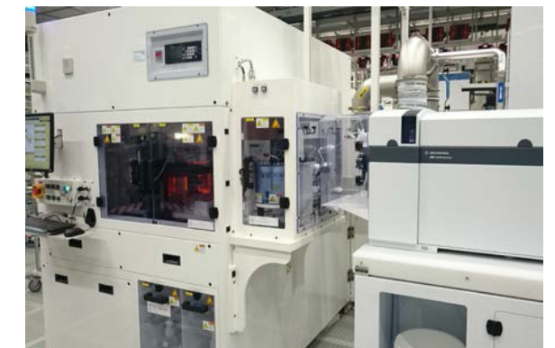
Expert PS fully automated VPD-ICP-MS system manufactured by IAS Inc. that was integrated with Agilent 8800 ICP-MS/MS. The figure was provided by ST Microelectronics (Crolles, France)
